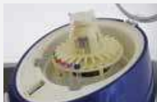
QuickPrep™ Sample Holder 24 x 2 mL tubes (included with FastPrep-24™ instrument) Cat. No. 116002512
